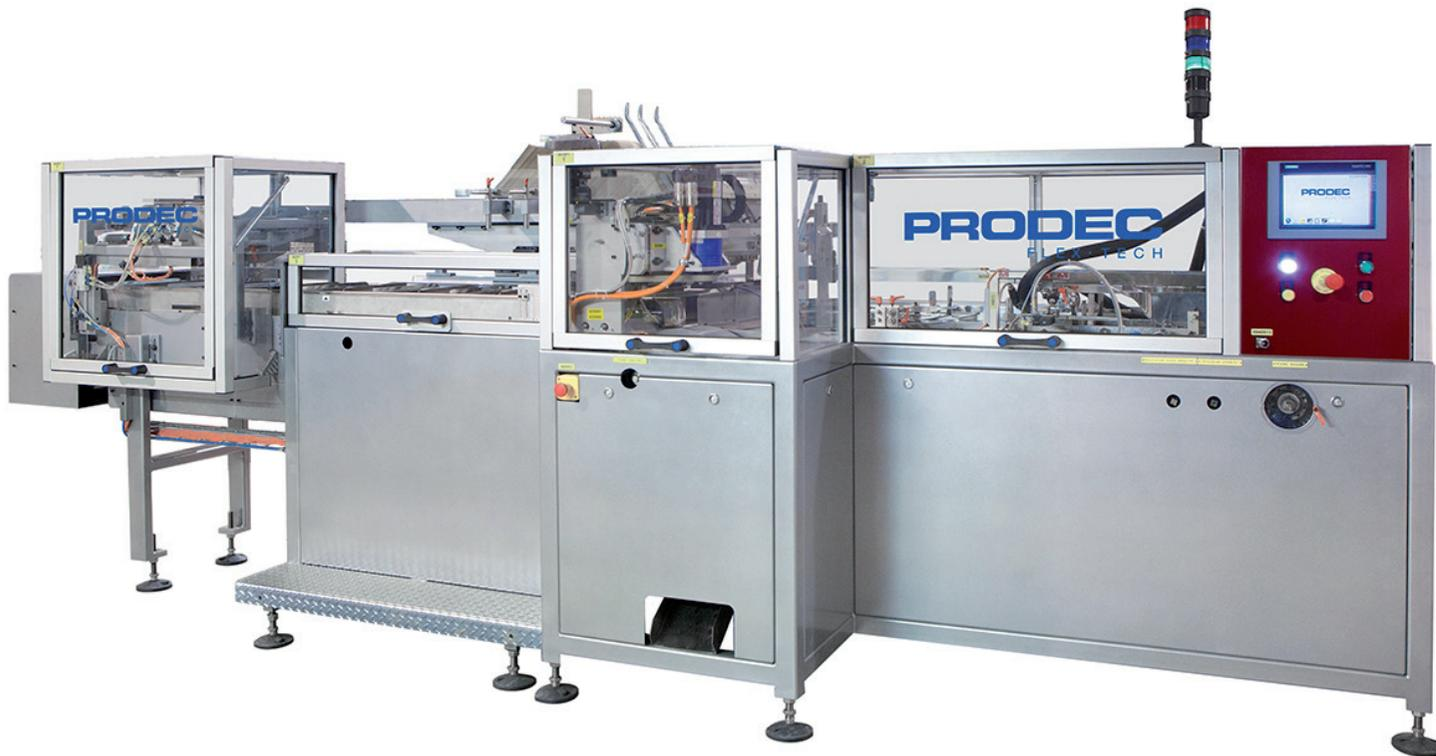
**ECI-20** is a compact and flexible side loading compact case packer with intermittent progress, for forming, filling and closing of cases in a single monoblock. The filling of cases is done by a pusher, adjusting speed according to product type, with expandable capacity depending on the required production output.
