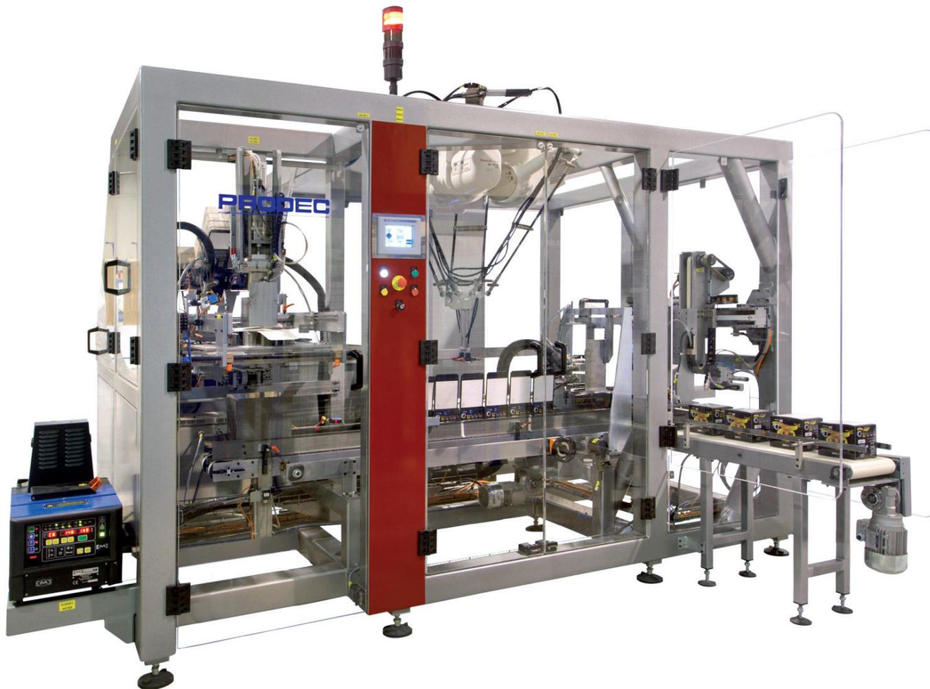
The **CP-101** is a top loading, compact and flexible case packer with Pick & Place cartesian system for forming, filling and closing cases or exhibitor cases in a single monoblock with. The filling of cases is performed by a pick & place mechanism with a simple gripping head with speed which is adjustable according to product type. The system is expandable depending on the required production output.
